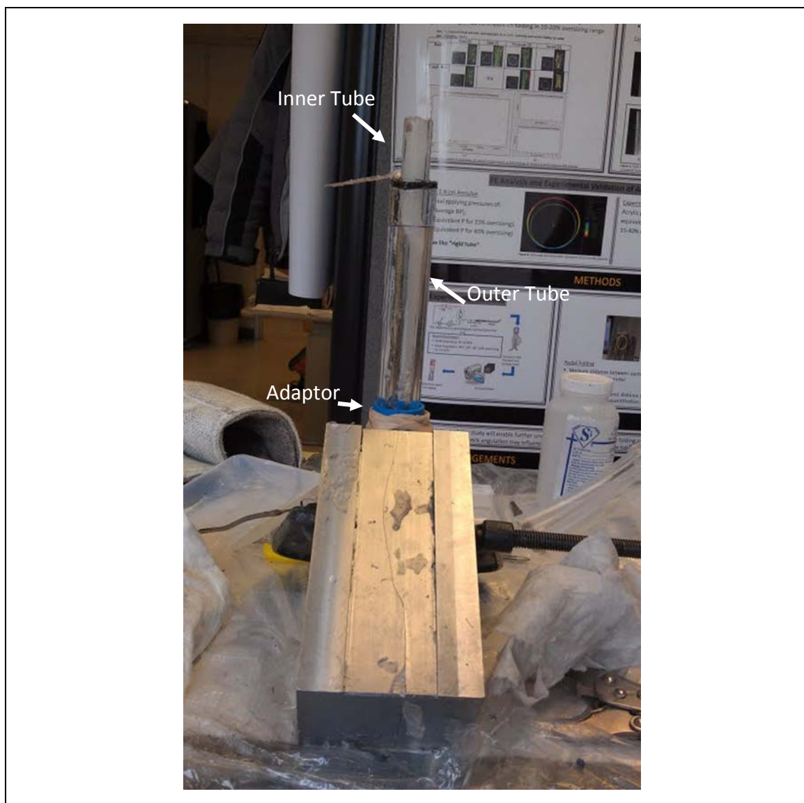
Figure 24: Clear acrylic pipes used as the silicone aorta mold. Two different aorta sizes with 19 mm (wall thickness 3.3 mm) and 25.4 mm ID (wall thickness 3.9 mm).
