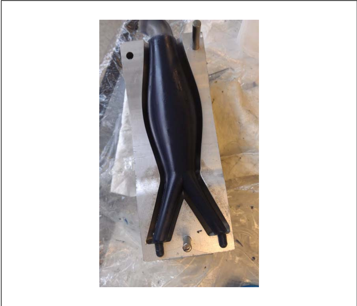
Figure 21: Placement of wax core into silicone mold milled from aluminum blocks. The gap between the wax core and aluminum mold will be filled with silicone. Thickness of the finished silicone model is the same as the gap between the wax and aluminum surface (4mm).
