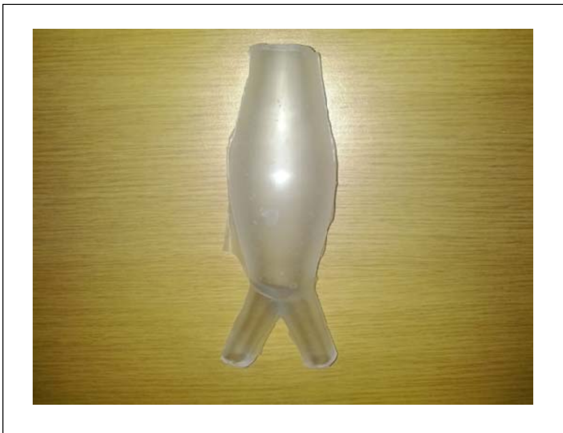
Figure 22: Finished transparent silicone AAA model with wall thickness of 4 mm.
